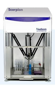
The Scorpion can access 6 deck positions with a minimal footprint. The unique lightweight and durable delta arm design allows for an open work space. The high speed arm movements increase throughput and facilitate the transfer of solvents without dripping. The enclosed work space can be filled with gas to create an inert environment.
