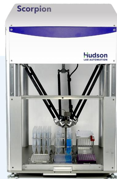
The Scorpion can access 6 deck positions with a minimal footprint. The unique lightweight and durable delta arm design allows for an open work space. The high speed arm movements increase throughput and facilitate the transfer of solvents without dripping. The enclosed work space can be filled with gas to create an inert environment.
